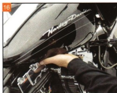
16 Continue routing the sensor wiring under the tank and up to the fairing.
