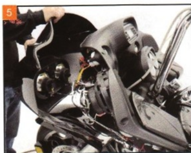
Remove the outer fairing and unplug the headlight wiring.
