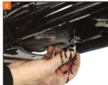
9 Remove the accessory plug from the oil pan.
