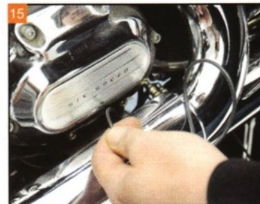
15 Route the sensor wiring to the battery box.
