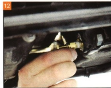
12 Install the temperature sensor into the adaptor.
