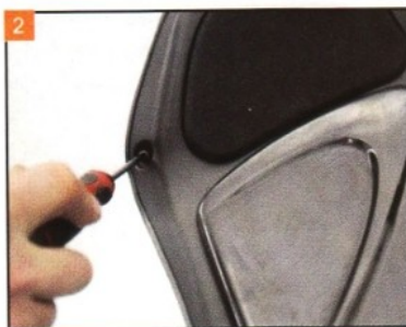
Remove the fairing mounting bolts.
