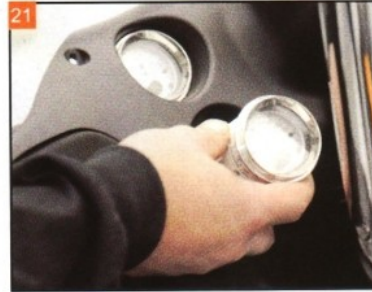
Remove the air temperature gauge.
