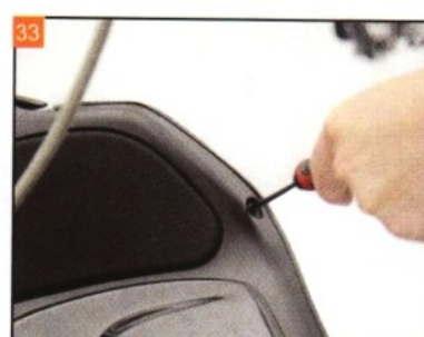
33 Install the fairing mounting bolts.
