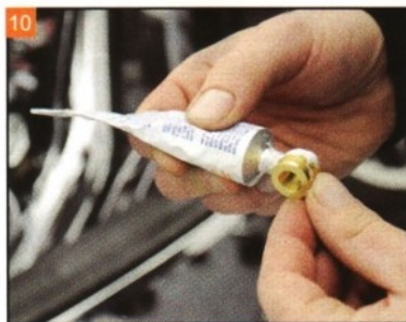
10 Apply thread sealant to the temp. sensor adaptor.
