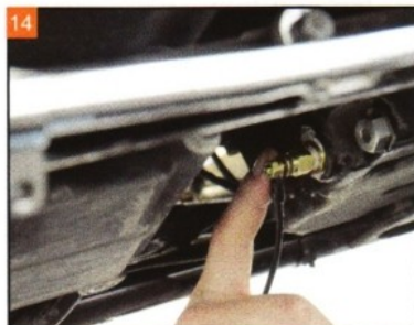
14 Install the sensor wiring and mounting hardware.
