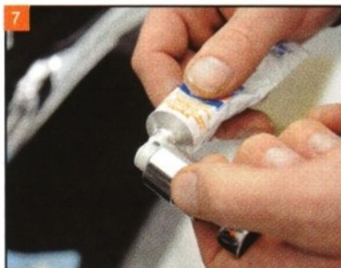
7 Apply thread sealant to the drain plug.
