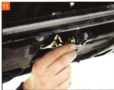
11 Install the adaptor into the oil pan accessory port.
