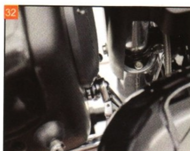
32 Install and tighten the turn signal mounting hardware.
