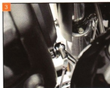
Loosen and remove the turn signal mounting hardware.
