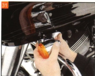
31 Install the turn signals through the fairing.
